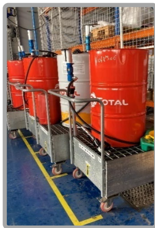
Storage of chemicals and paint on retention tanks (equipped room or tanks)
